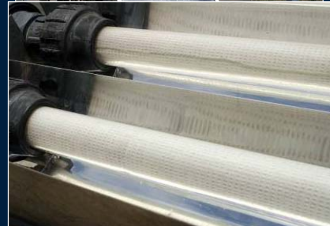
Reactor CPC (soporte coaxial)
